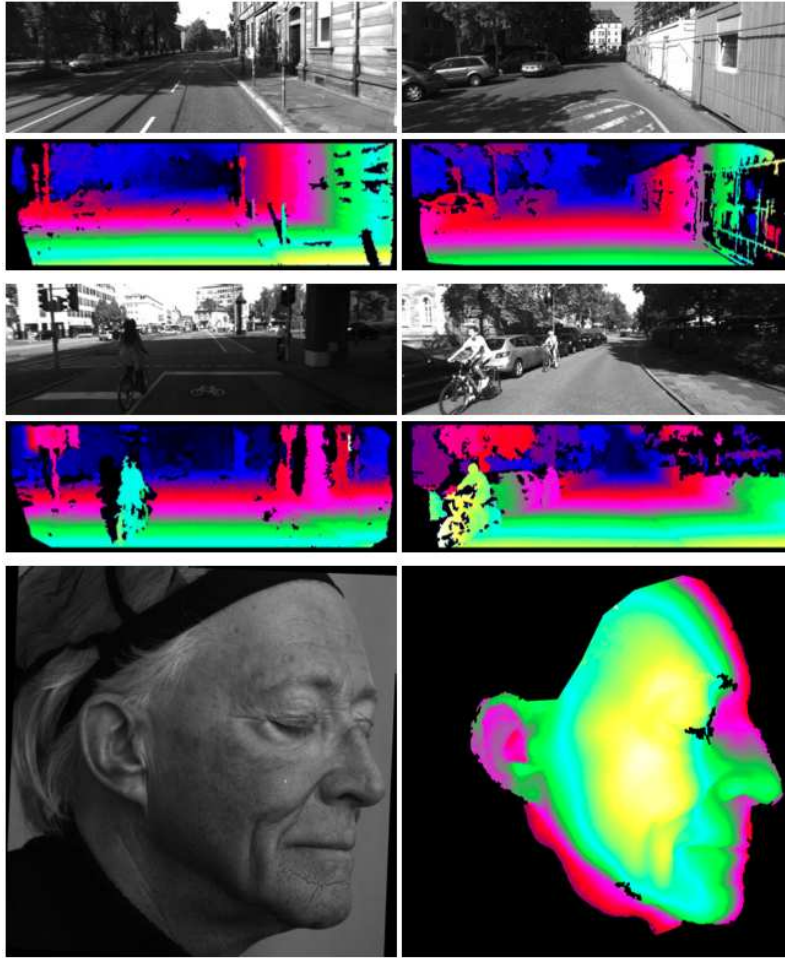
Figure 4.2.: Results of the ELAS stereo reconstruction on an urban video sequence and a face image. (Source: [GRU11])
