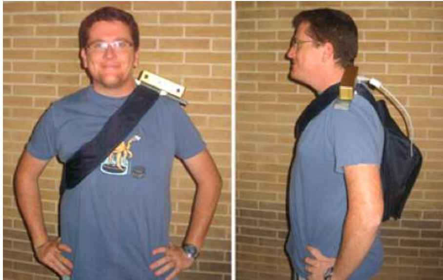
Figure 2.2.: A wearable stereo device for aerial obstacle detection. It is comprised of a Bumblebee stereo camera and a laptop. (Source: [MR + 08])
