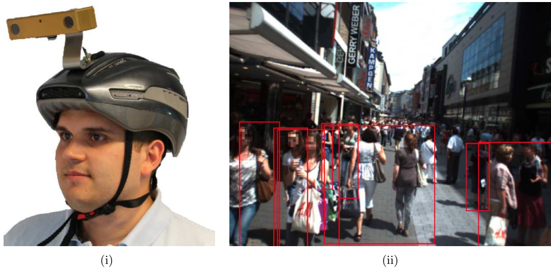
Figure 2.4.: Close Range Human Detection for Head Mounted Cameras. The left image (i) shows the setup which consists of a Bumblebee camera mounted to a helmet. In the right image (ii) detections of humans in a pedestrian area can be seen. (Source: [ML12])
