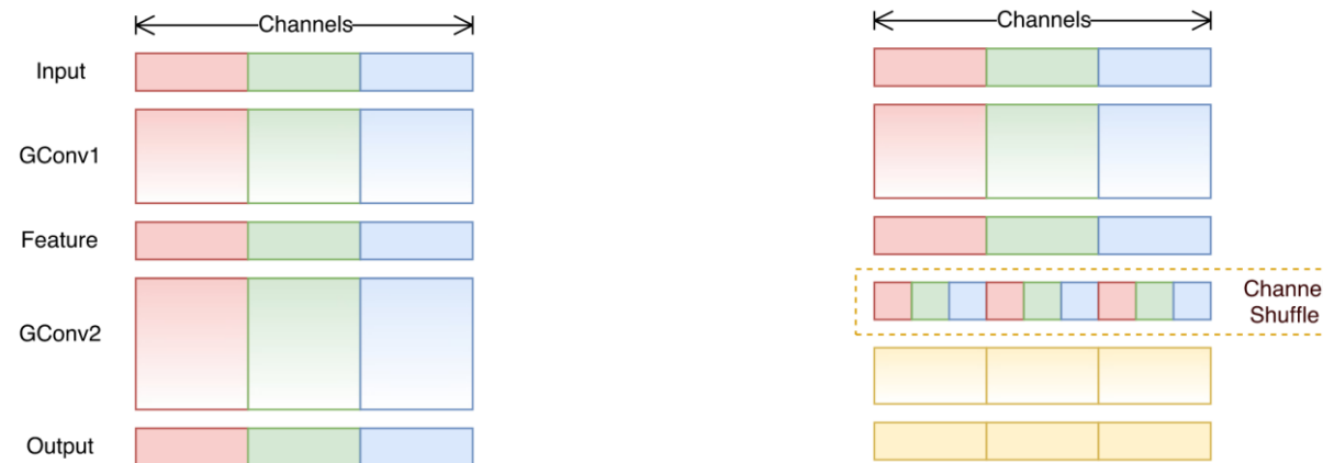
Visualization of the grouped convolution problem and its solution
