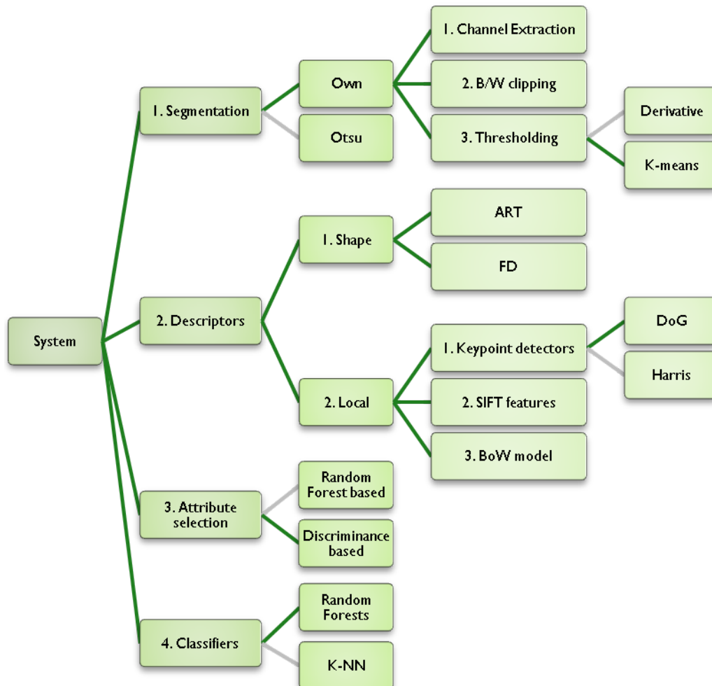
Figure 4.2: Overview of the possible configurations of the system. Numbered cases represent steps, unnumbered cases represent choices. The grayed links represent implemented and tested elements which are however not part of the best and final system configurations.
