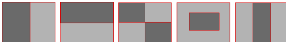
Figure 1: Example Haar-like features consisting of two, three and four base rectangles.
